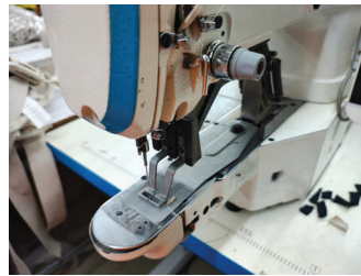
Eye guards were missing of eyelet machine at sewing section.jpg
