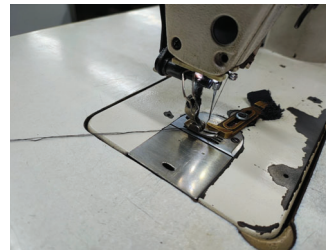
Needle guard of sewing machines were displaced condition.jpg
