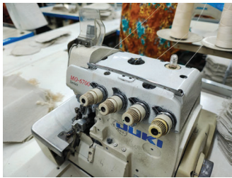
Eye guards were displaced of overlock machine at sewing section.jpg
